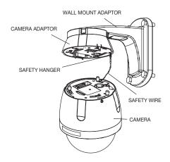
13. Align the Guide 1 of the Camera with the Guide 2 of the Camera Adaptor and insert the 3 Guides of the Camera into the corresponding Guide Holes of the Camera Adaptor. Then, turn the camera clockwise by 10 degrees.
